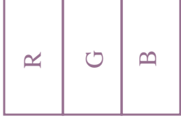
new HIRES mosaic detector layout: 3 2048x4096 CCDs
